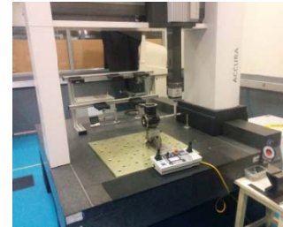
Fig. 2: Set – up in CMM for crankcase
